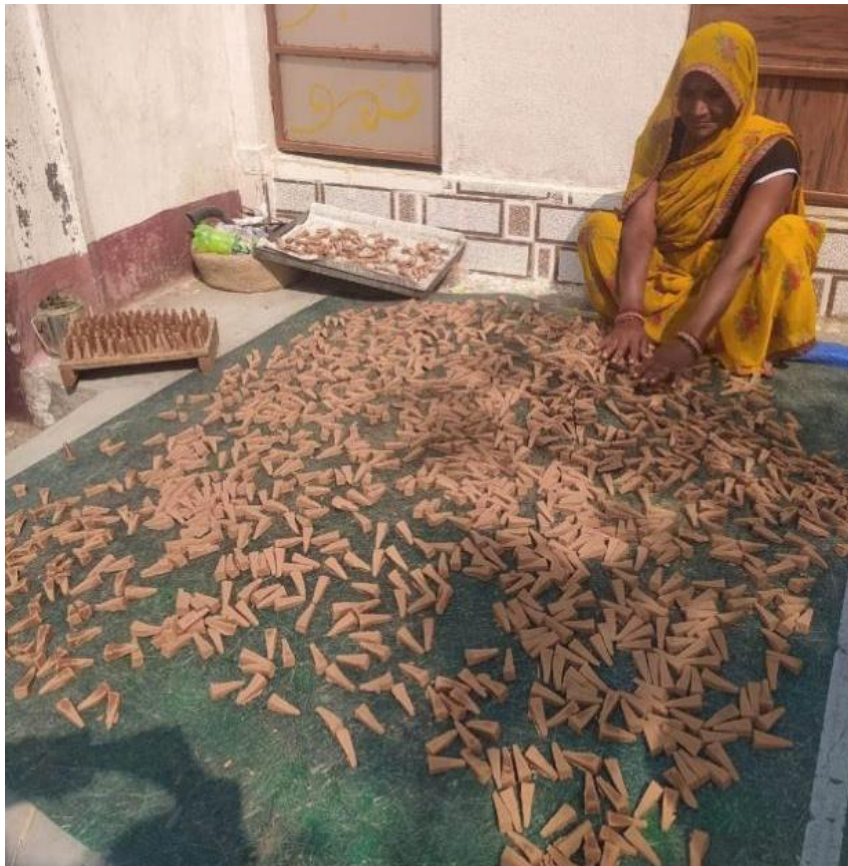
Figure 7: Sun drying process of Dhoopbatti and Agarbatti
